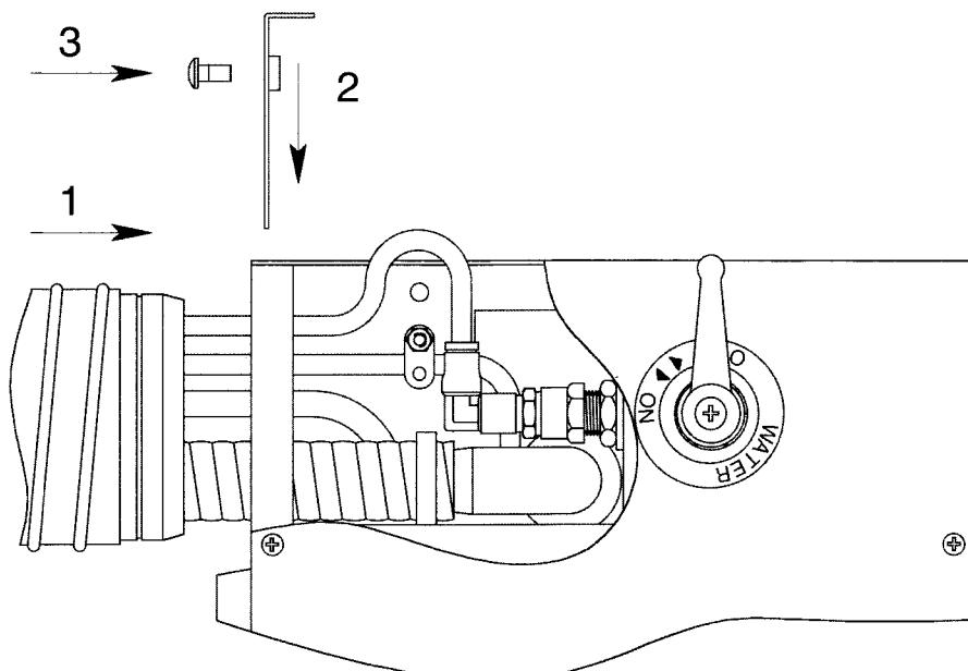
Connect up the services using the fittings supplied, do not use the small grey waste elbow to connect Dry-line suction hose as this will restrict the air flow.
