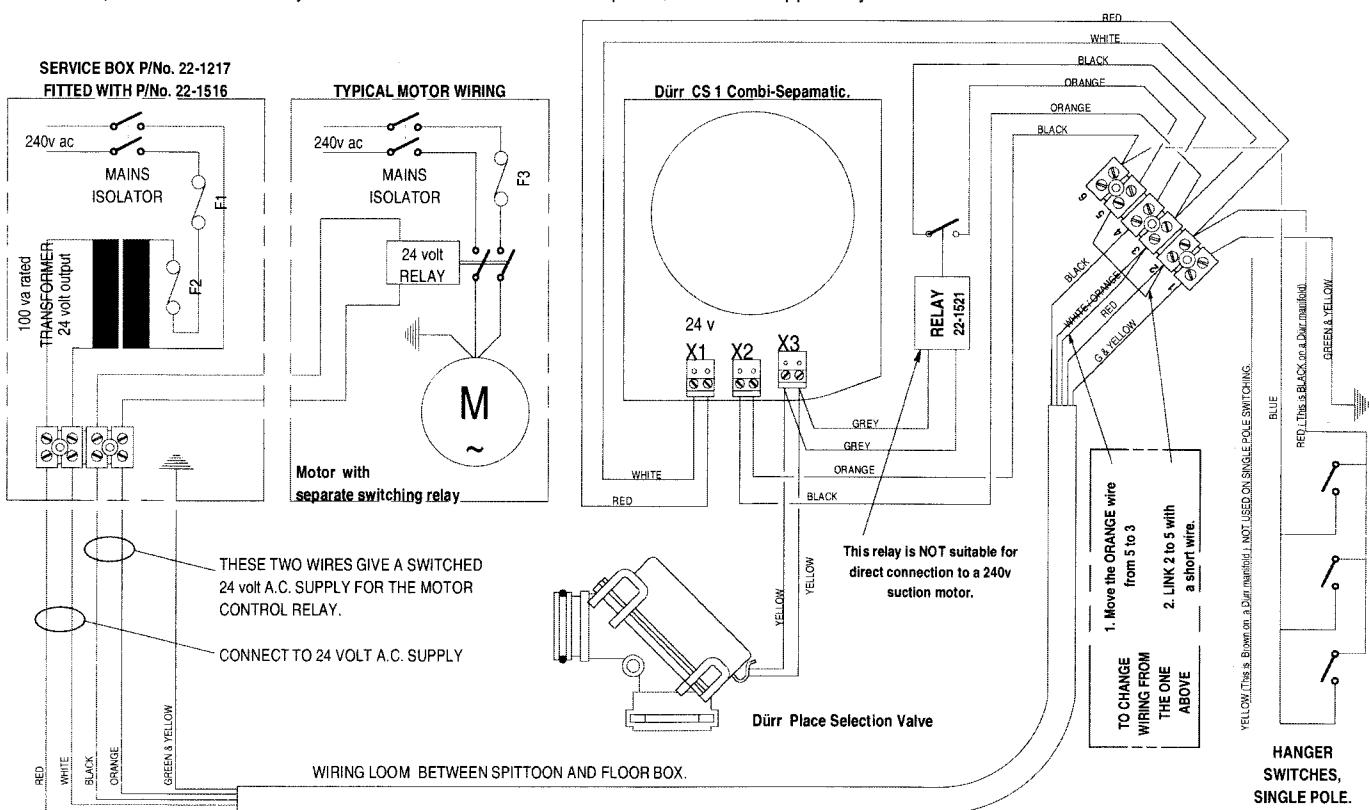
**WIRING CONNECTIONS FOR CS 90 SPITTOON, model 90CA**
