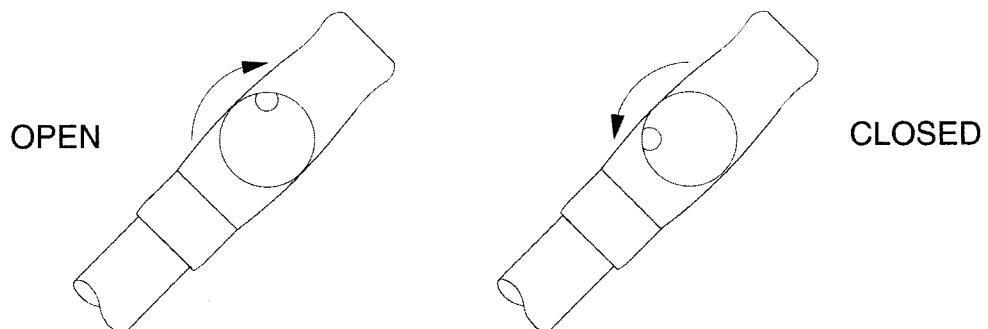
Since the control of vacuum is by occluding the suction bores, the equipment is only suitable for use with motors/suction pumps which are safe to run 'shut-off' or which incorporate vacuum relief devices.
