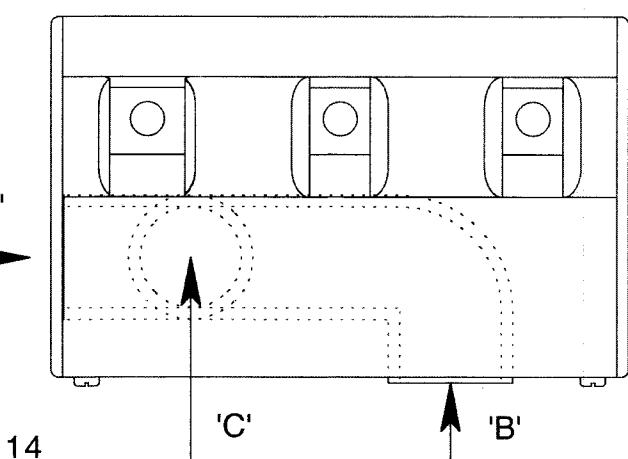
To gain access, the spittoon door panel will need to be removed. Undo the screw at the base of the spittoon, as indicated below, until it clears the hole in the door panel. Move the bottom of the panel slightly outwards, then remove by pulling downwards.
