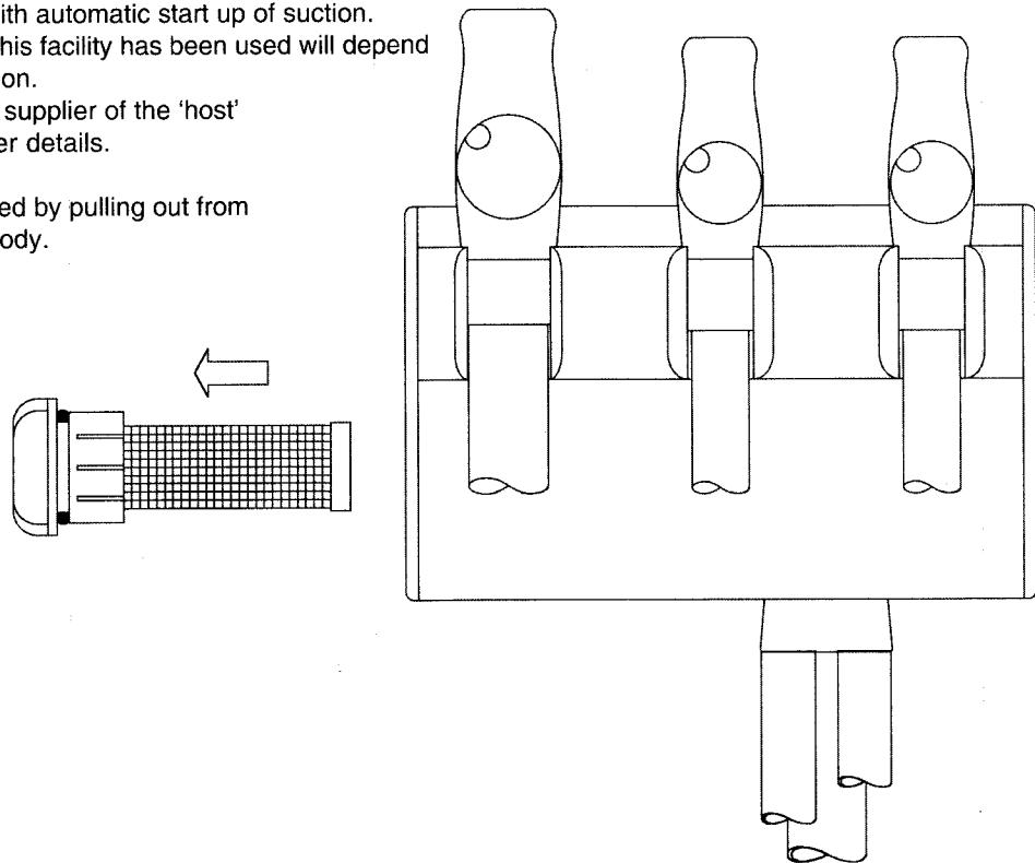
Lifting one of the hoses from its holder will result in automatic start up of suction. The degree of suction is varied by rotary action valves incorporated in the cannula connectors, as shown below. Moving the valve anti-clockwise, as indicated by the arrow, results in a reduction of suction. When the nodule is at its lowest position, suction is virtually shut-off.
