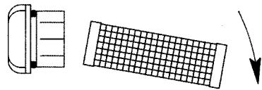
Remove the sleeve by tilting gently to the side and pulling. Use only moderate force to avoid damaging the holder.
