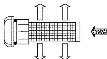
Note that air flow is in to the open end and out through the surface as indicated by the arrows. Thus brushing the mesh from the outside will displace trapped debris. After cleaning, the 'O' ring seal should be lubricated with a little silicone grease.
