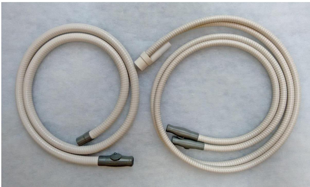
A modified manifold connector with a plug-on 14mm operating hose significantly reduces the vacuum level needed to produce a 300 litre/minute air flow rate. Indicative testing \* revealed a vacuum level of 70 mbar at the back of the manifold connector @ 300 l/min.
